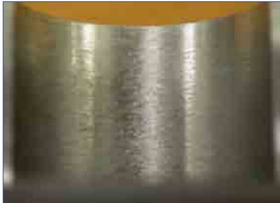
Drilled with HP at V=1150 sfm
