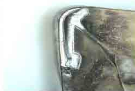
CNMG432MT TT8115 After 300 linear inches
