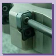
\*Tighten the insert screw completely (35in. lbs.)
