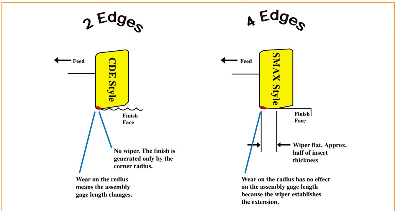
It is clear from the above figures that the wiper flat on the end of the SMAX 18 MM insert is a significant design enhancement for the Maxline product line. This new face mill series allows us to give our customers the combination of “tangential” insert orientation strength, true square shoulders when necessary, and the consistent finishes that result from a ground wiper flat on the inserts.
